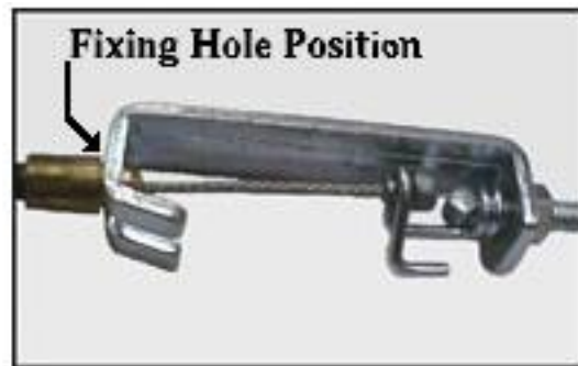
Step d. Fix the salience of the copper end Of the upper cable into the fixing hole of the joint bracket.
