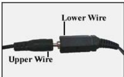
Step e. Connect the upper computer wire with the lower computer wire. Push together to be whole piece.
